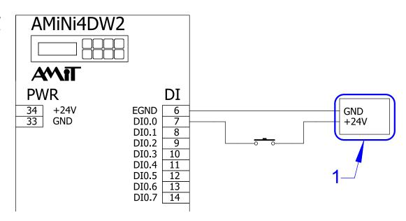
Fig. 7 - Passive contact supplied from individual power supply
