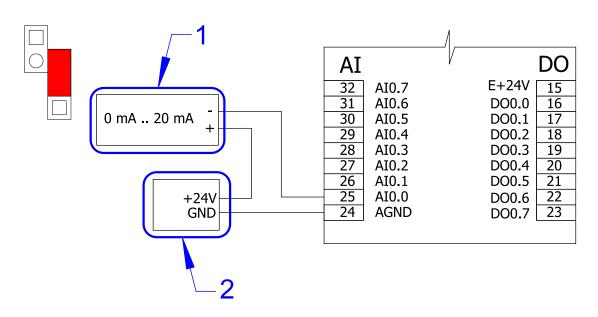
Fig. 21 - Connecting sensor with current output 0 mA to 20 mA (4 mA to 20 mA)
