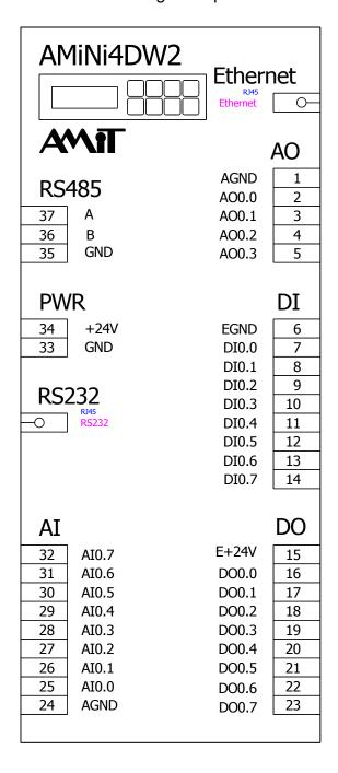
Fig. 2 - Recommended drawing symbol for AMiNi4DW2
