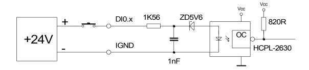
Fig. 6 - Wiring scheme of single digital input channel
