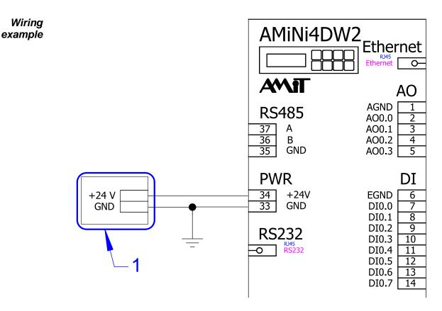
Fig. 4 - Wiring example of single control system
