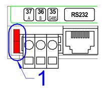
Fig. 29 - Connected jumpers on end station
