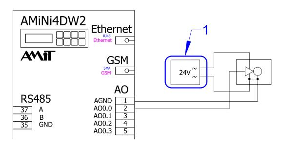
Fig. 25 - Connecting AC supplied servo
