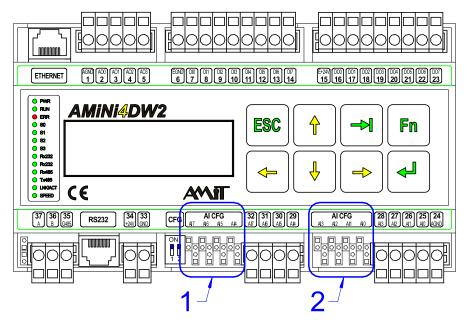
Fig. 18 - Configuration jumpers location
