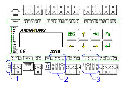
Fig. 34 - Configuration jumpers location
