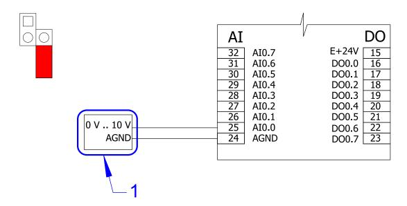
Fig. 20 - Connecting voltage sensor 0 V to 10 V
