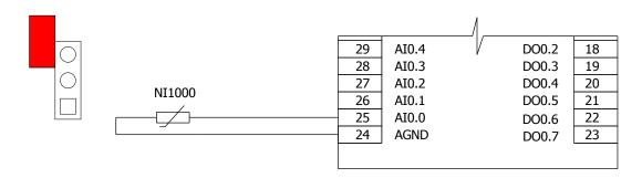
Fig. 22 - Connecting Ni1000 sensor
