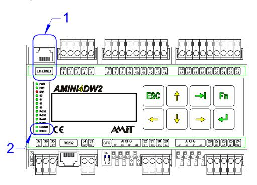
Fig. 31 - Ethernet connector and indication LEDs location
