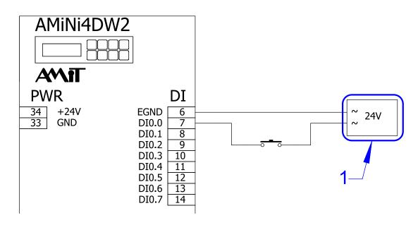
Fig. 9 - Passive contact supplied from AC power supply
