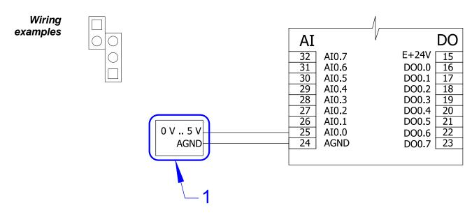
Fig. 19 - Connecting voltage sensor 0 V to 5 V
