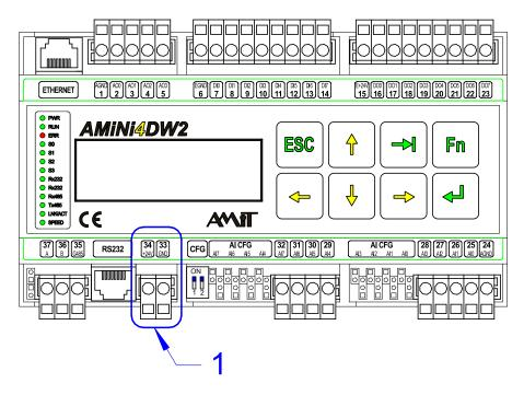
Fig. 3 - Power supply connector location
