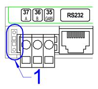
Fig. 30 - Disconnected jumpers on end station
