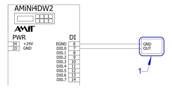
Fig. 8 - Connecting self-supplied active output
