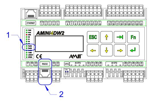
Fig. 26 - Connector and indication LEDs location
