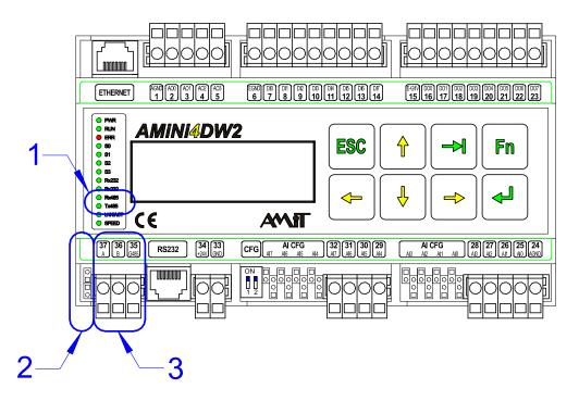
Fig. 28 - RS485 connector and indication LEDs location
