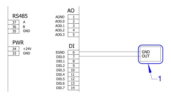
Fig. 8 - Connecting self-supplied active output
