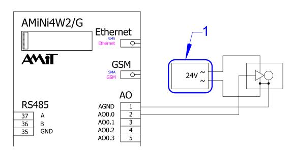
Fig. 25 - Connecting AC supplied servo
