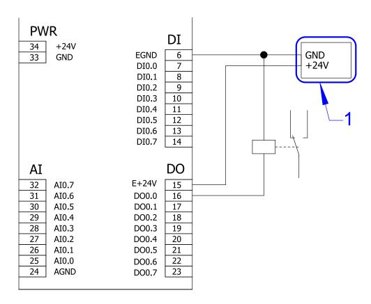
Fig. 11 - Operating the power contactor by semiconductor output
