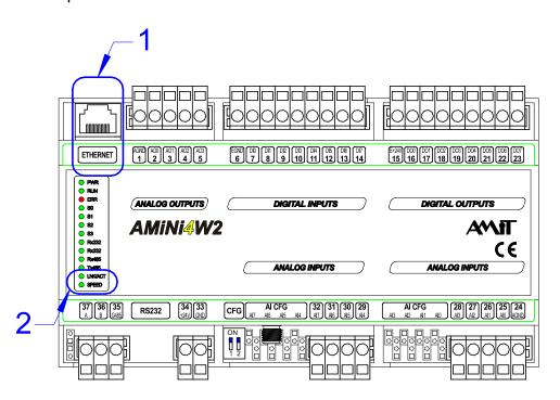
Fig. 29 - Ethernet connector and indication LEDs location
