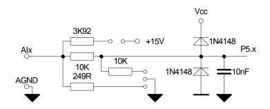
Fig. 13 - Wiring scheme of analogue input single channel
