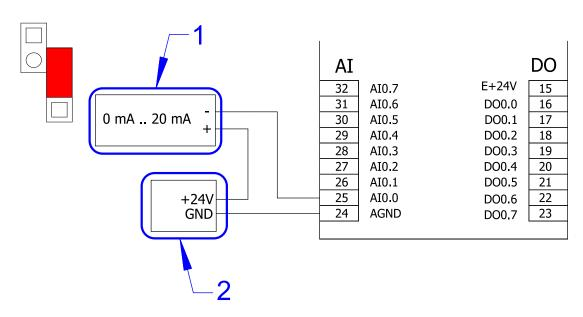
Fig. 21 - Connecting sensor with current output 0 mA to 20 mA (4 mA to 20 mA)
