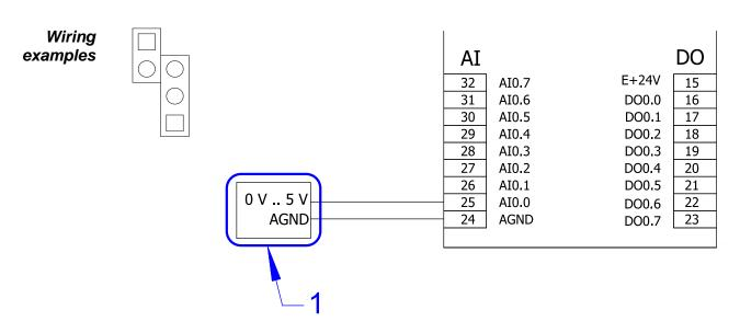
Fig. 19 - Connecting voltage sensor 0 V to 5 V
