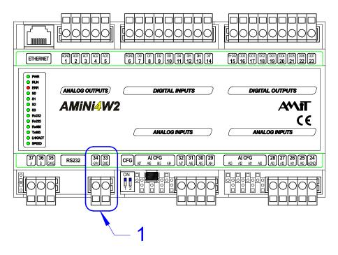
Fig. 3 - Power supply connector location
