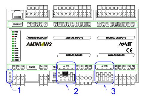
Fig. 34 - Configuration jumpers location
