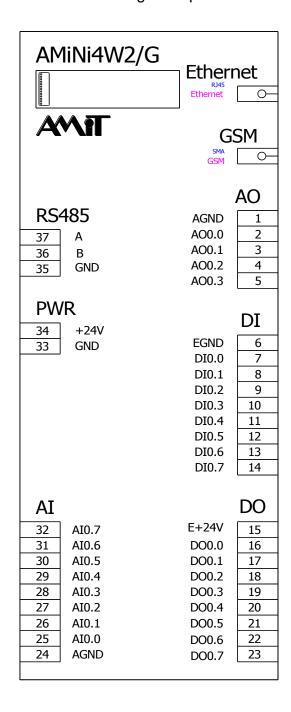
Fig. 2 - Recommended drawing symbol for AMiNi4W2/G
