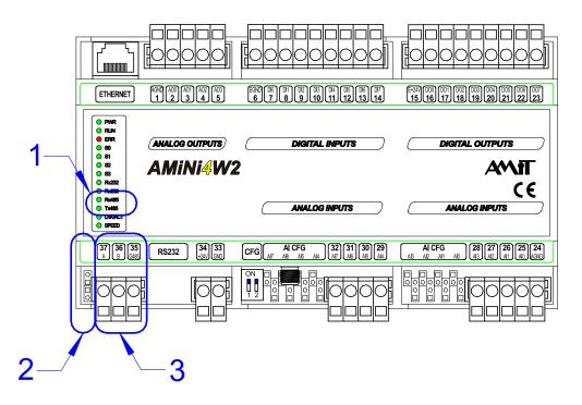
Fig. 26 - RS485 connector and indication LEDs location
