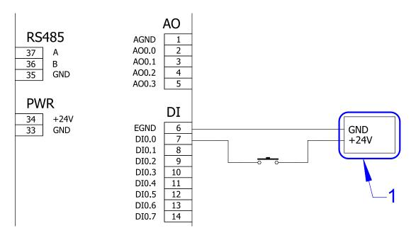
Fig. 7 - Passive contact supplied from individual power supply
