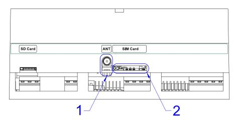
Fig. 30 - Antenna connector and slot for SIM card location
