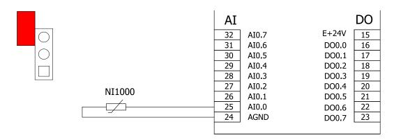
Fig. 22 - Connecting Ni1000 sensor
