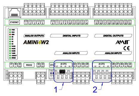
Fig. 18 - Configuration jumpers location
