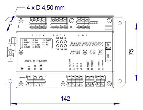
Fig. 17 – Dimensions of mounting holes
