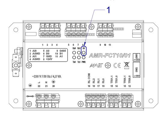
LED S0 serves for indication of a module software application state.
