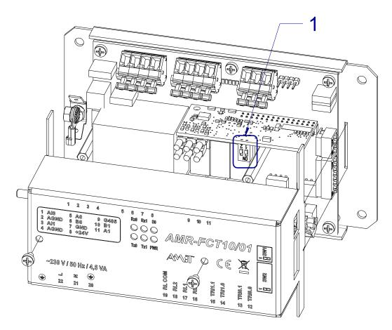
Fig. 20 - Service DIP switch location
