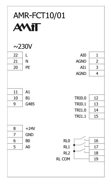
Fig. 2 – Recommended drawing symbol for **AMR-FCT10/01**
