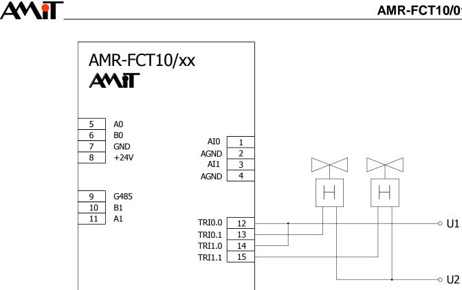
Fig. 16 - Triac output wiring example
