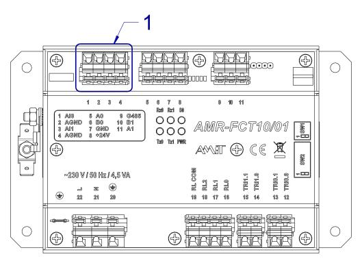
Fig. 10 - Location of terminals for RTD inputs
