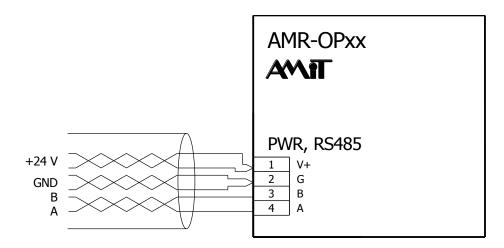
Fig. 8 – Structured cabling use example
