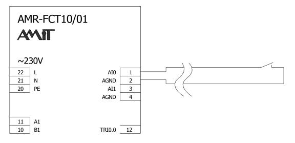
Fig. 12 – Dry contact wiring example
