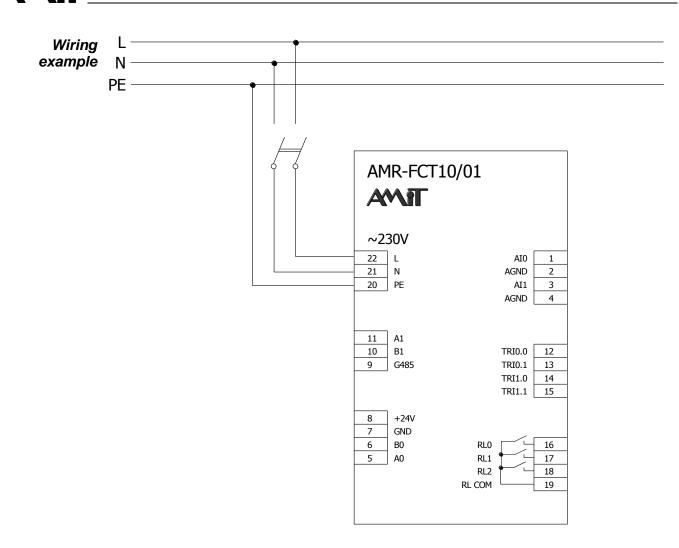
Fig. 4 – Power supply wiring example
