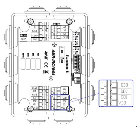
Fig. 12 - Digital output terminals location
