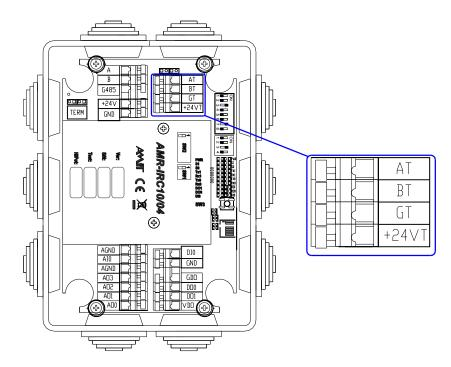
Fig. 15 – RS485 interface terminals location
