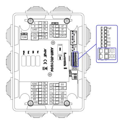
Fig. 13 - Location of digital output status LEDs
