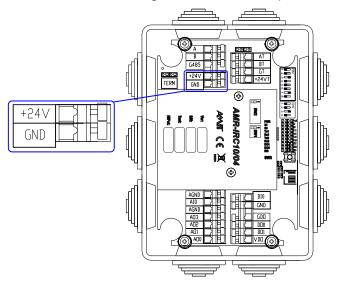
Fig. 3 – Power supply terminals location
