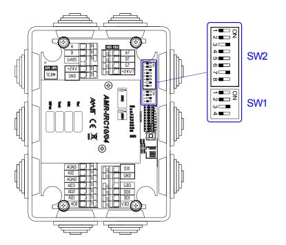
Fig. 24 - Configuration DIP switches location
