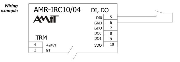
Fig. 11 – Example of contact wiring to DI0
