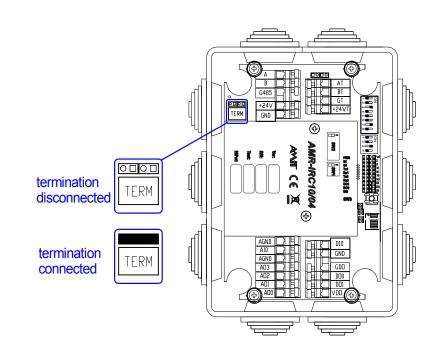
Fig. 20 - RS485 configuration jumpers location (COM1)
