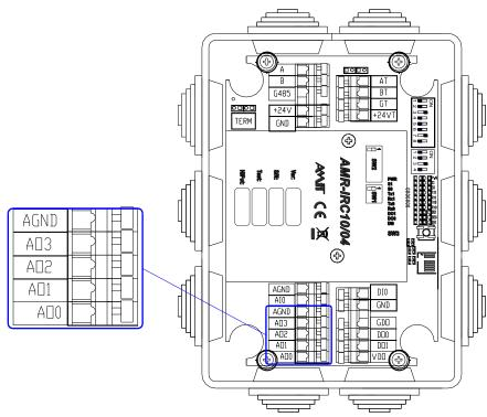
Fig. 7 – Analogue output terminals location
