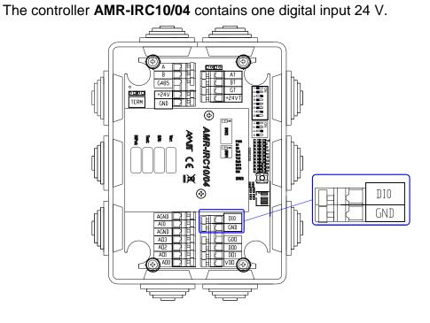
Fig. 9 – Digital input terminals location
