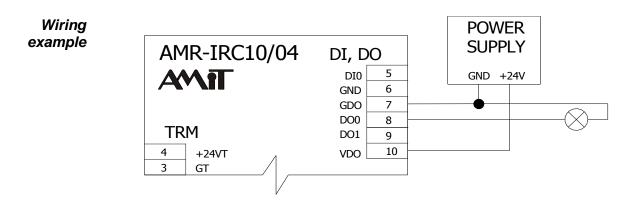
Fig. 14 - Signal light wiring to DO0 output
