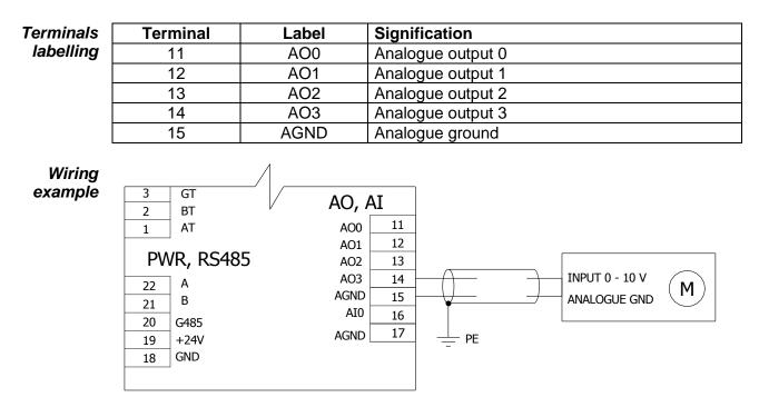
Fig. 8 – Example of wiring a drive to AO3 analogue output
