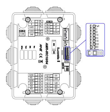
Fig. 10 - Digital input status LEDs
