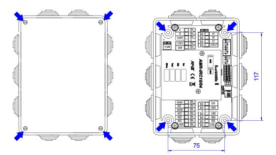
Fig. 23 - Unit cover removal, mounting hole dimensions
