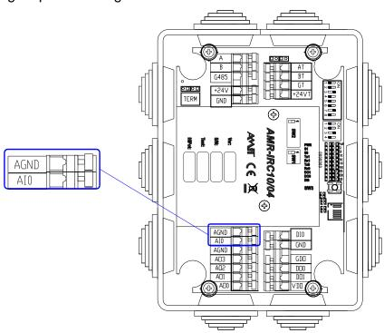
Fig. 5 – Analogue input terminals location
