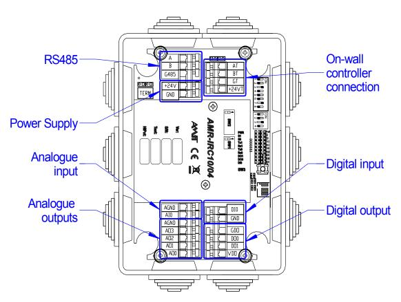
Fig. 21 – Connector location
