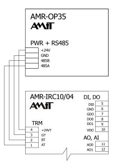
Fig. 17 – Wiring example of the room controller AMR-OP35
