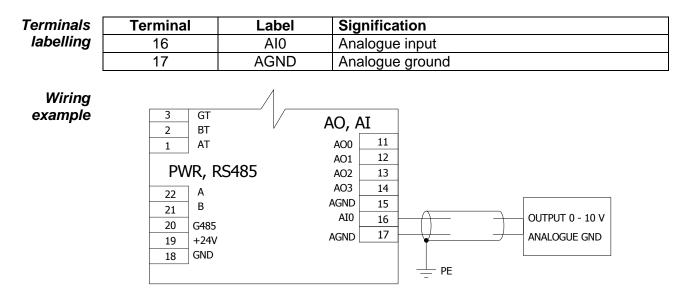
Fig. 6 – AI wiring example
