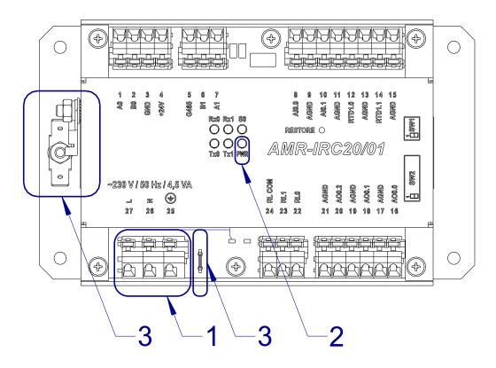
Fig. 3 – Terminals location for power supply
