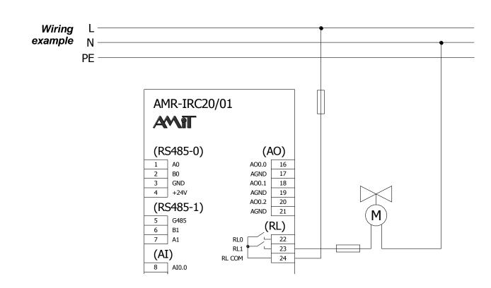
Fig. 18 – Wiring example of thermoelectric head connection to relay output
