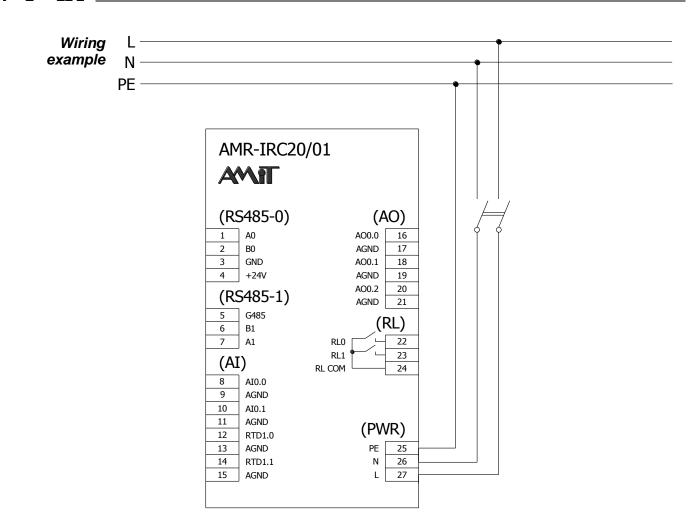
Fig. 4 – Power supply wiring example
