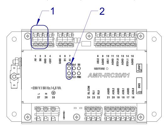
Fig. 5 – Terminals and LEDs location for RS485 without GI
