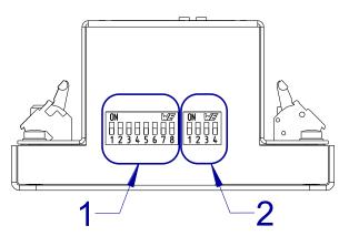
Fig. 19 - DIP switch location for communication parameters setting
