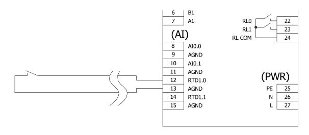
Fig. 14 – Dry contact wiring example
