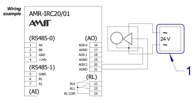
Fig. 16 - Wiring example of servo connection with AC voltage power supply
