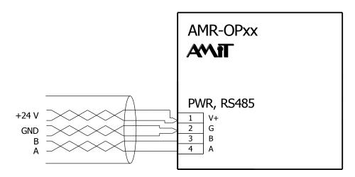
Fig. 8 – Structured cabling use example
