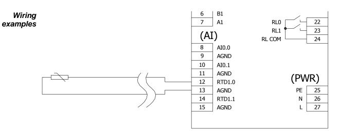
Fig. 13 – Temperature sensor wiring example
