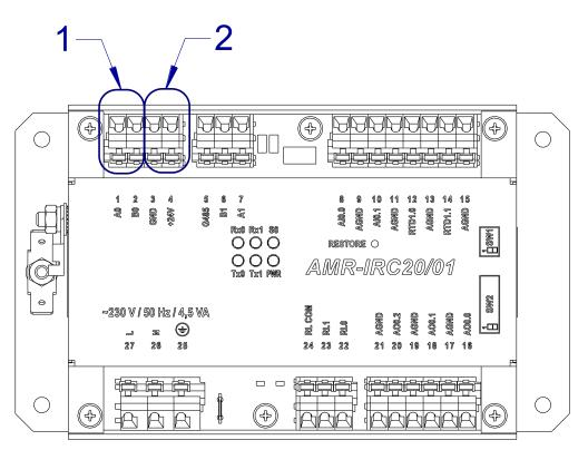
Fig. 6 – Terminals location for on-wall controller connection
