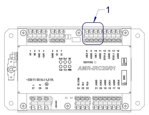
Fig. 10 – Terminals for analogue input
