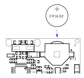
Fig. 11 - Battery insertion
