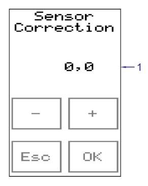
Fig. 30 - Correction of temperature sensor
