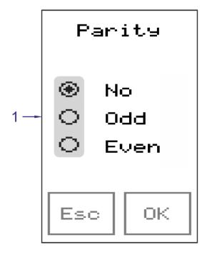
Fig. 35 - Setting parity for MODBUS protocol
