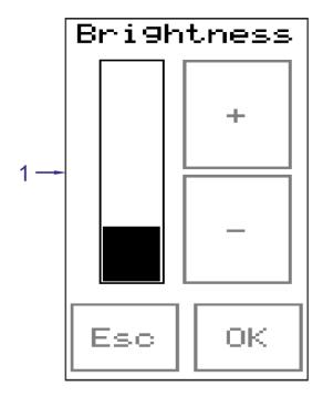
Fig. 22 - Brightness adjustment
