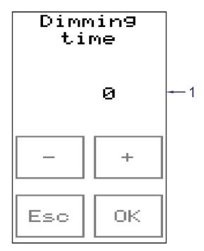
Fig. 25 - Setting time for screen saver activation
