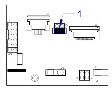
Fig. 38 - Interconnection of service jumper on AMR-OP70B/xx PCB
