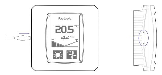
Fig. 10 - Place, that must be pressed with flat screwdriver
