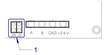
Fig. 8 - RS485 configuration jumpers location
