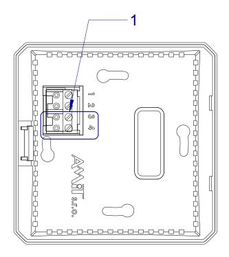
Fig. 5 - RS485 connector location
