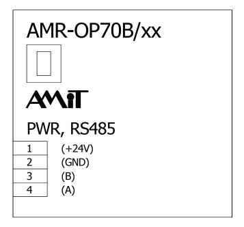
Fig. 2 - Recommended drawing symbol for AMR-OP70B/xx
