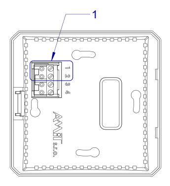
Fig. 3 - Power supply connector location
