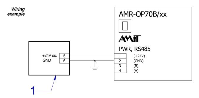
Fig. 4 - Power supply wiring example
