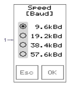
Fig. 34 - Setting communication speed
