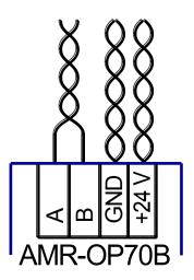
Fig. 7 - Connecting structured cabling to terminals of the controller
