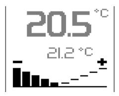
Fig. 16 - Correction of required temperature
