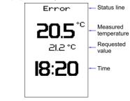
After the first touch of the screen - backlight is turned on, after the second touch - basic screen is displayed.
