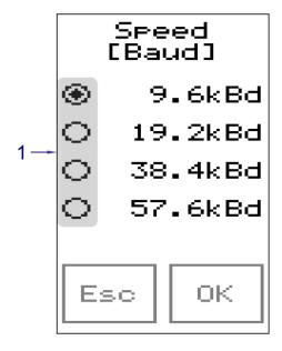
Fig. 31 - Setting communication rate
