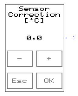
Fig. 35 - Correction of temperature sensor
