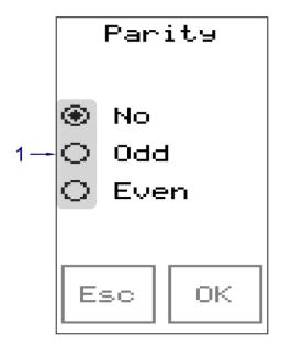
Fig. 32 - Setting parity for MODBUS protocol
