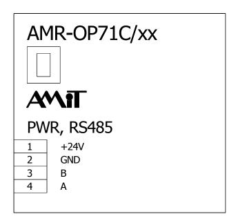
Fig. 2 – Recommended drawing symbol for AMR-OP71C/xx
