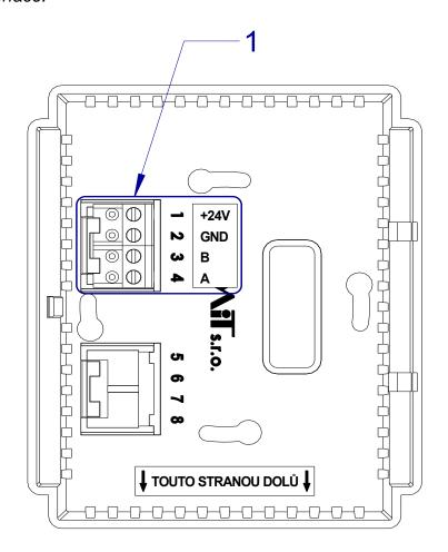
Fig. 3 – Power supply connector location
