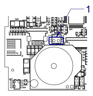
Fig. 45 – Interconnection of service jumper on AMR-OP71C/xx PCB
