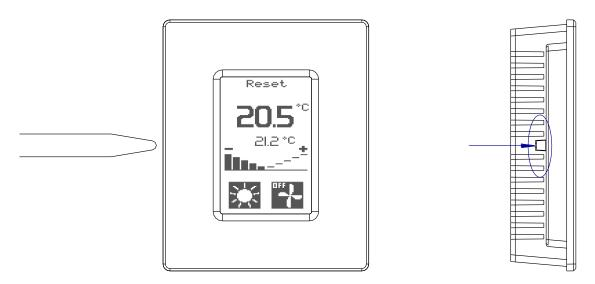
Fig. 8 – Place that must be pressed with blunt-tip
