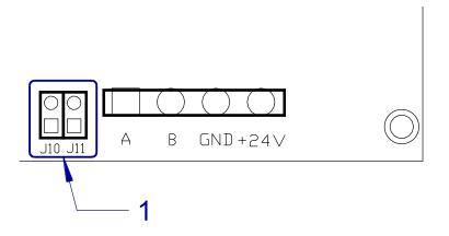
Fig. 5 – RS485 configuration jumpers location
