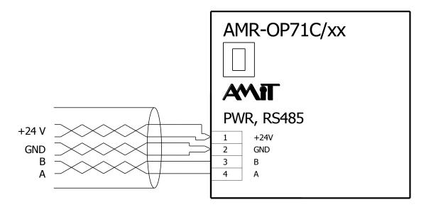
Fig. 6 – Example of structured cabling usage
