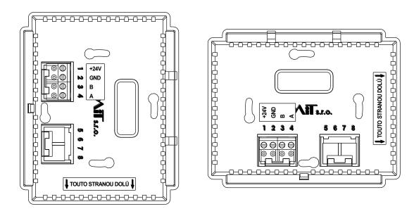
Fig. 7 – On-wall controller mounting in vertical position (left), in horizontal position (right)
