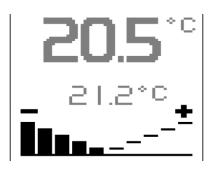
Fig. 13 - Correction of required temperature
