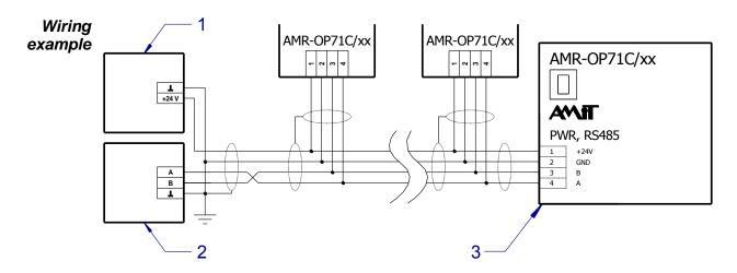
Fig. 4 – Power supply and RS485 wiring
