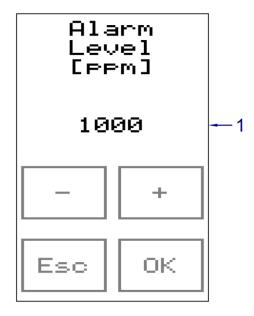
Fig. 36 - CO<sub>2</sub> concentration for acoustic warning
