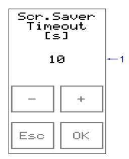
Fig. 24 - Setting time for screen saver activation
