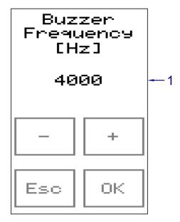
Fig. 41 - Frequency of acoustic warning
