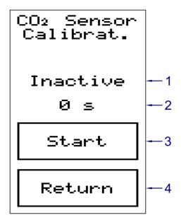
Fig. 37 – Manual CO<sub>2</sub> sensor calibration
