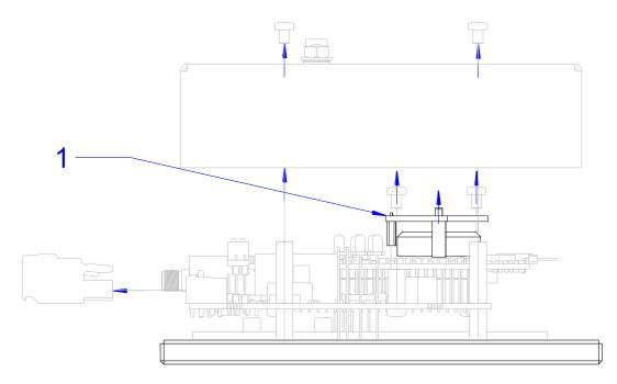
Fig. 19 - Ejecting battery module
