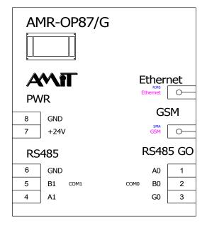
Fig. 3 - Recommended drawing symbol for AMR-OP87/G
