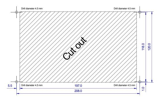
Fig. 12 - Mounting apertures
