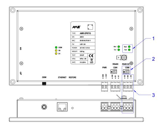
Fig. 6 - Location of galvanically separated RS485 connector
