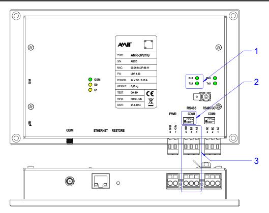
Fig. 7 - Location of RS485 line connectors
