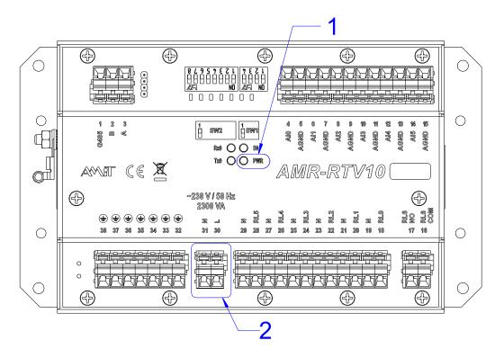
Fig. 3 – Power supply terminals location
