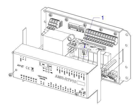
Fig. 15 - Service DIP switch location
