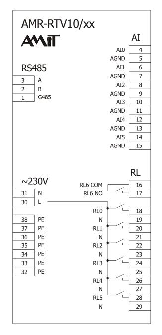
Fig. 2 – Recommended drawing symbol for AMR-RTV10/01
