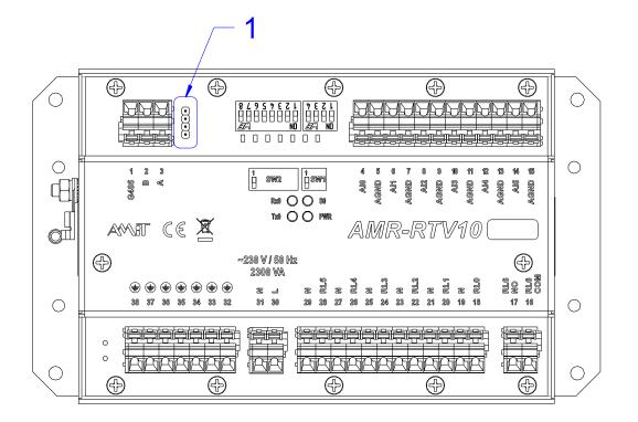
Fig. 10 - RS485 configuration jumpers location
