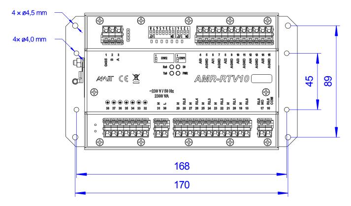
Fig. 12 – Dimensions of mounting holes
