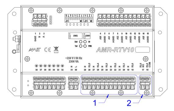
Fig. 7 - Relay outputs terminals location
