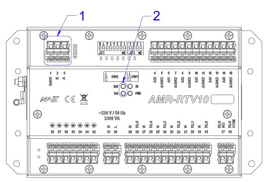
Fig. 9 - RS485 interface terminals location
