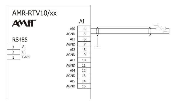
Fig. 5 - Ni1000 / Pt1000 sensor wiring example
