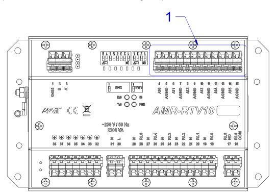
Fig. 4 – Universal input terminals location
