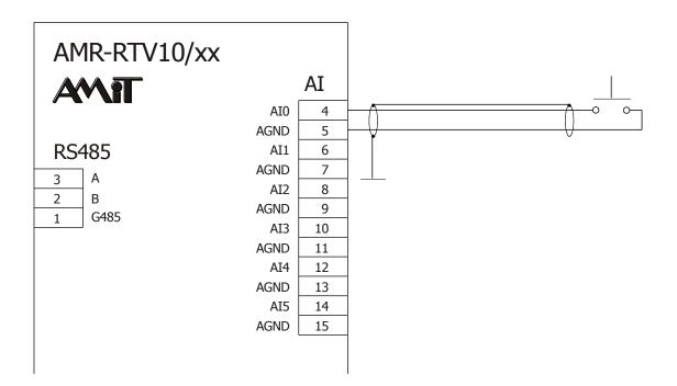
Fig. 6 – Dry contact wiring example
