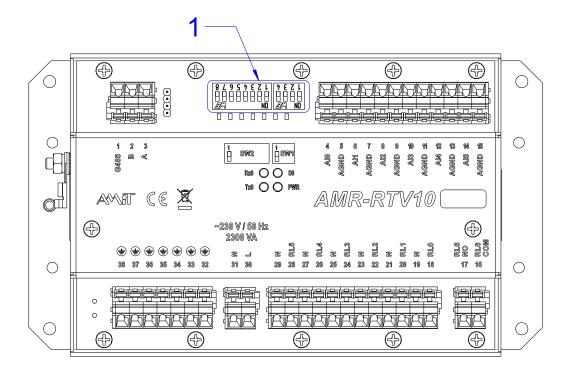
Fig. 14 - Location of configuration DIP switches
