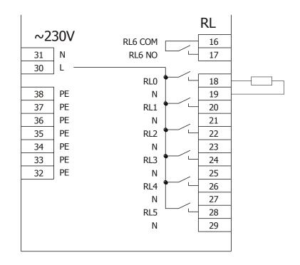
Fig. 8 - Relay output wiring example
