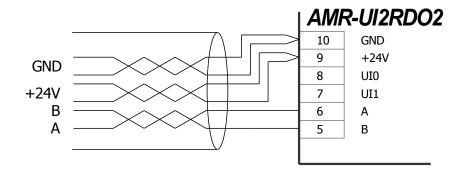
Fig. 5 - Example of use of structured cabling
