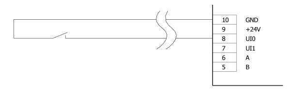
Fig. 8 - Potential-free contact wiring example
