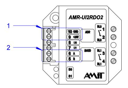
Fig. 3 - Location of power supply and RS485 terminals
