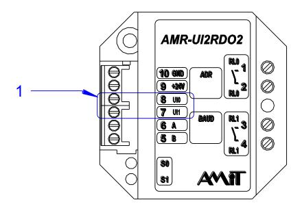
Fig. 6 - Location of universal inputs terminals
