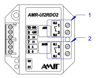
Fig. 9 - Location of relay outputs terminals
