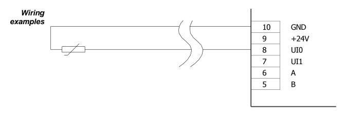
Fig. 7 - Example of temperature sensor connection
