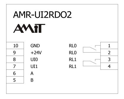
Fig. 2 - Recommended drawing symbol for **AMR-UI2RDO2**
