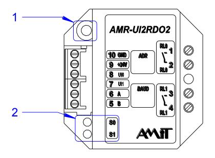
Fig. 10 - Location of indication LED's and service button
