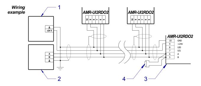
Fig. 4 - Power supply and RS485 wiring
