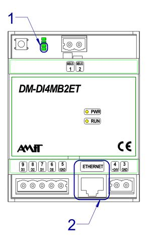
Fig. 11 - Location of LEDs and connector for Ethernet
