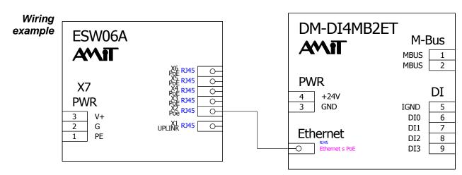
Fig. 5 – Example of power supplying from power supply PoE
