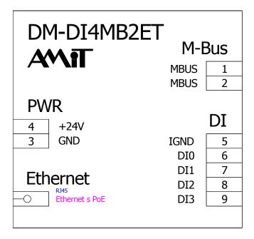
Fig. 2 – Recommended drawing symbol for **DM-DI4MB2ET**
