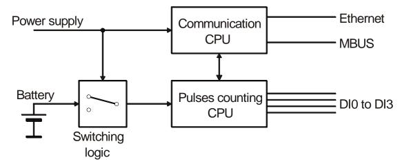
Fig. 8 – Block scheme of internal wiring
