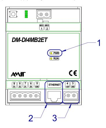
Fig. 3 – Power supply connector +24 V DC
