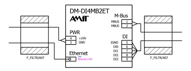
Fig. 13 - Ferrite filters wiring on the cables
