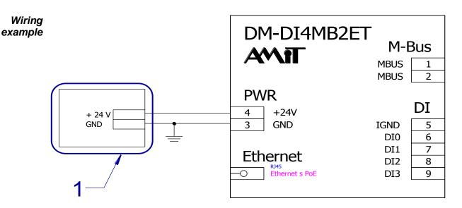
Fig. 4 – Example of power suppling from power supply +24 V DC
