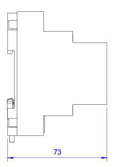
Fig. 1 – **DM-DI4MB2ET** dimensions
