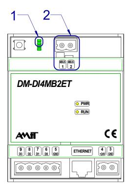
Fig. 9 – Location of LEDs and terminals for M-Bus
