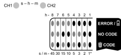
peated brief presses of the PROG button. Time of closing can be set in the following values: 2, 3, 5, 10, 15, 30, 45 s, 1, 2, 3, 5, 10, 15, 30, 45 min and 1 to 8 h. Press (long press) the PROG button to return to the operation mode.
